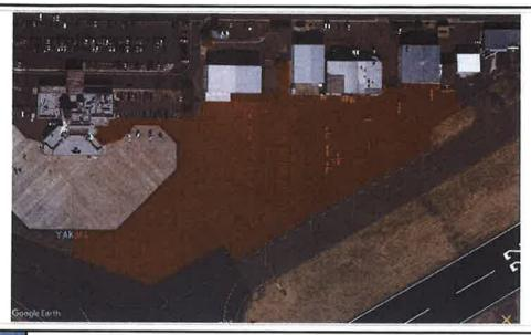
The East Ramp supports general aviation (GA), business, Part 121, and Part 135 operators. The existing asphalt is deteriorating. It is severely cracked and weathered with a PCI index ranging from 25 to 55. The East Ramp needs major rehabilitation.
