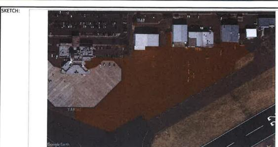
The East Ramp supports general aviation (GA), business, Part 121, and Part 135 operators. The existing asphalt is deteriorating. It is severely cracked and weathered with a PCI index ranging from 25 to 55. The East Ramp needs major rehabilitation.
