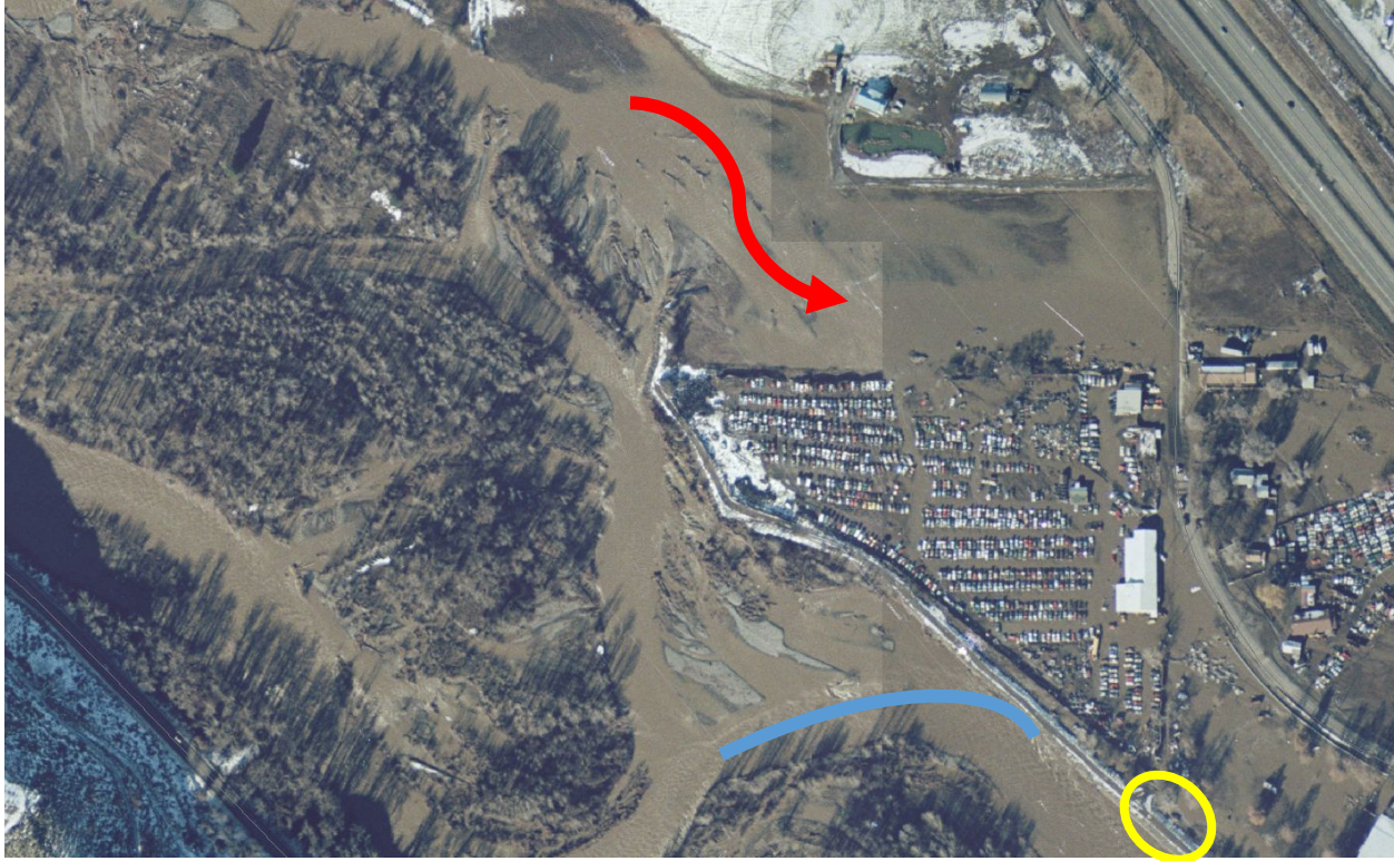
Figure 6 – 1996 Flood 2 days after 50-year peak flow, river is at about 25-year flow in photo. Red arrow shows flanking path upstream of Ramblers’ Park levee, Corps and County extended the levee 450 feet upstream in the ensuing weeks. Just above the blue line in the development of the “jet” as the flow falls, area where the “jet” hits the levee would fail and collapse 3 days later. Yellow circle is second failure, approximately a month later as the “jet” reformed downstream. Note also the fresh gravels depositing upstream of the blue line, along the red line and continuing upstream off the photo.
