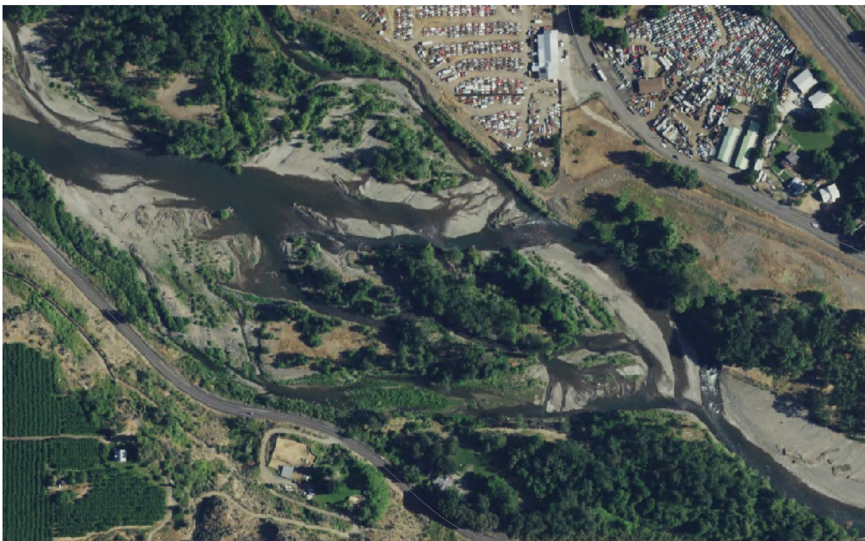
Figure 22 – Aggraded Bar, Ramblers’ Park 2017, after construction of 3 pilot channels in late 2015. Note increase in wetted channel area and diversity.
